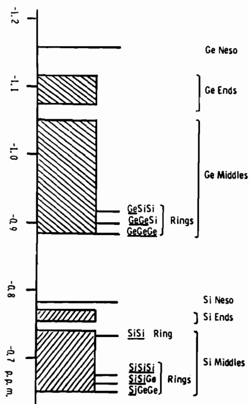
Figure 1. Schematic proton NMR spectrum of equilibrated mixtures in the system (\text{CH}_3)_2\text{SiCl}_2 - (\text{CH}_3)_2\text{GeCl}_2 - [(\text{CH}_3)_2\text{SiS}] - [(\text{CH}_3)_2\text{GeS}] referenced to internal tetramethylsilane.
